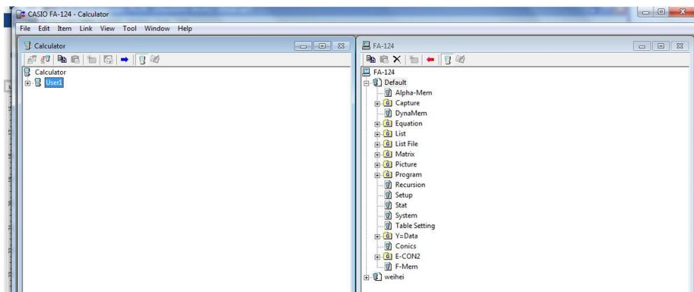
**Note:** Each Folder is a capture of all files in each of the **MAIN MENU** icons on the hand-held FX9750Gii calculator. Dragging folders or files from the right screen to the left screen will transfer files from the laptop/PC to the hand-held FX9750GII.
