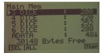
Review what file(s) to be transmitted by selecting them with the **[EXE]** key to open the folder, scroll through the files using the **▲** or **▼** arrows, and press **[F1]** to select the file and a **▶** will appear on the left of the file name. When the files have been selected, press **[F6]** to transfer these to the receiving calculator.
