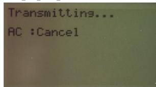
A 'Transfer Completed' message will appear on both screens when the file transfer is completed. Follow the instructions on the 'Receiving calculator' and if you want to send the same files to another calculator (e.g. a class set), then press **[F2]** for **CuRreNT**, and **[F6]** for transmitting, otherwise press **[EXIT]** to escape or **[MENU]** to return to the **MAIN MENU**.
