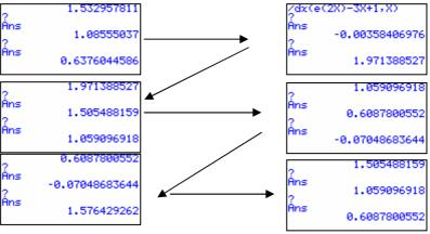
You can see that the iteration method 'osculates about and does not settle onto a solution.
