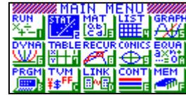
select GRAPH mode from the main menu by using the arrow keys to highlight the GRAPH icon or pressing 5.
